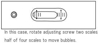
(iv) A pattern where the zero points of neither level nor surface plate are adjusted
