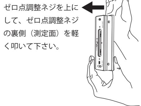
Tap lightly on the other side of measurement, placing up the adjustment screw.
