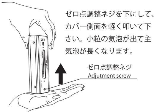
Tap lightly on the side of its cover, placing down the adjustment screw. Small bubbles would appear and the main bubble would be longer.
